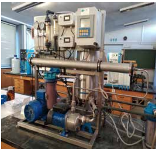
Fig.1. Laboratorial facility of reverse osmosis used in the experiments.
