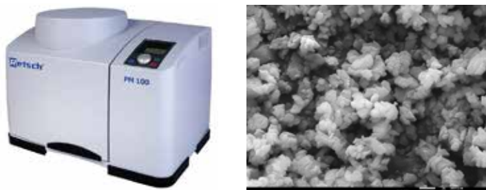
Fig.1. Left: Planetary Ball Mill; Right: SEM image of CaO Catalyst before reaction
